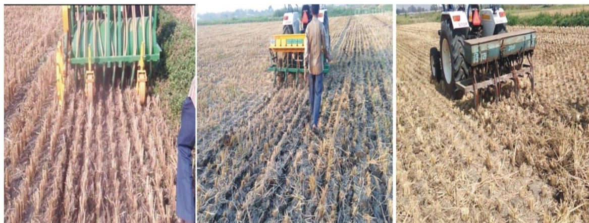
Figure. 1 Sowing of chickpea with T 1 , T 2 and T 3 machine under heavy stubbles of rice
